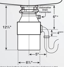
Distance from bottom of sink to center line of disposer outlet. Add 1/2" when stainless steel sinks are used.
