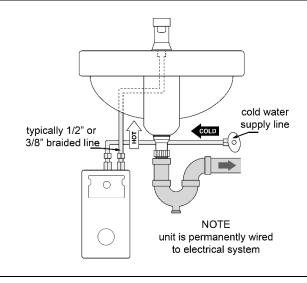
**4.** Open the hot water faucet and run water for a minimum of 60 seconds and until the flow is continuous and free of air pockets. Close the faucet and install the aerator (if supplied).
