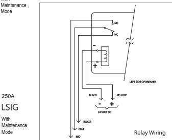
15. This feature allows enabling of the maintenance mode remotely by applying 24 vdc to the yellow (+) and black(-) wires that exit the left hand side of the breaker. The maintenance mode settings that is enabled is the 2.5x setting.
