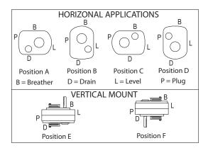
Figure 3 - Mounting Positions
