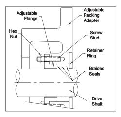
Figure 2 - Optional Adjustable Packing Adapter
