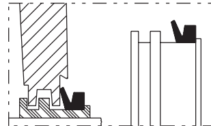
TRIPLE-TECT Seal General purpose seal for wet or dirty environments
