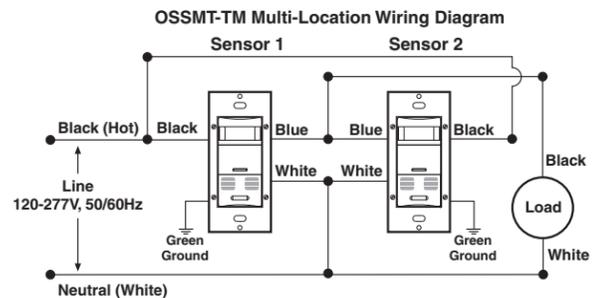
NOTE: Sensor 1 must be installed in a wall box that has both a LINE Hot and a Ground connection. Sensor 2 must be installed in a wall box that has both a Load and a Ground connection. If you are unsure about any part of these instructions, consult an electrician.
