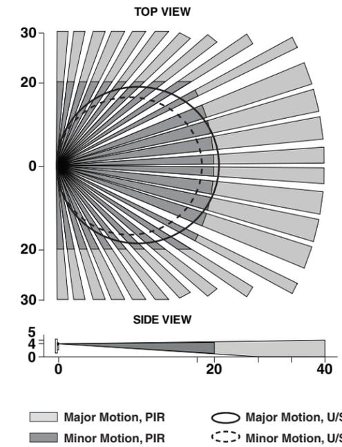
**Minor Motion = Dual Technology coverage.** This also represents the maximum ultrasonic range coverage.
