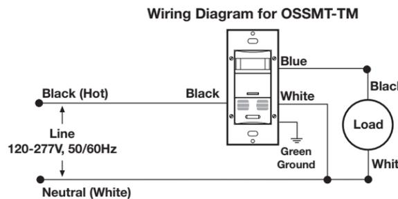
**WIRING SENSOR:** Connect wires per WIRING DIAGRAM as follows: Screw wire connector on clockwise making sure there are no bare conductors below the wire connectors. Secure each connector with electrical tape.
