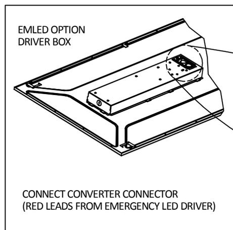
MAKE SUPPLY CONNECTIONS THROUGH ACCESS PLATE PROVIDED ON TOP OF THE LUMINAIRE. (SEE FIGURE-2)
