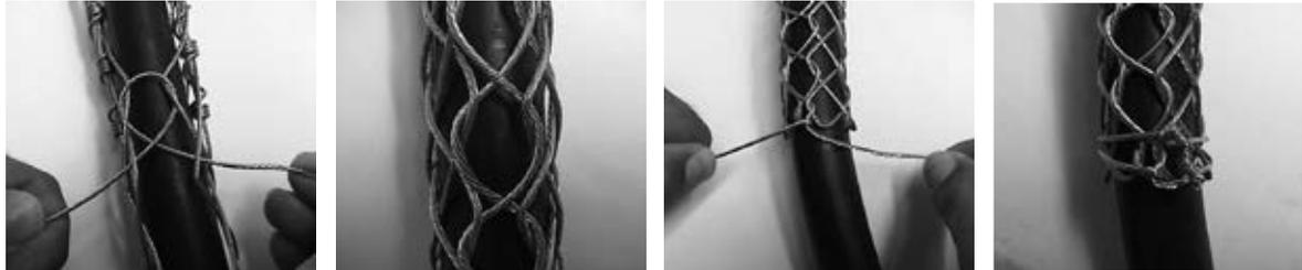
1. Place the grip around the cable. Starting at the eye end, thread the lace through the first two loops on either side of the mesh split. Pull the lace through the loops until the lace strands and thread them through the next two loops. Continue lacing the grip with this method
