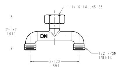
DIMENSIONS ARE IN INCHES AND [MILLIMETERS].
