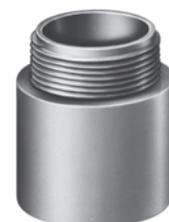
For adapting nonmetallic conduits to boxes threaded fittings, metallic systems. Male threads on one end, socket end on other.
