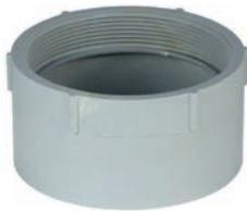
For adapting nonmetallic conduits to threaded fittings, metallic systems. Female threads on one end, socket end on other.
