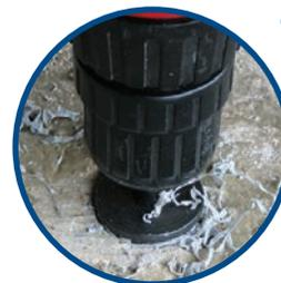
**4.** The guide will direct the cutter; the stop will touch when completed.
