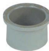
Adapts nonmetallic conduit to all electrical enclosures by inserting adapter through knockout and cementing into Carlton couplings.
