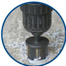
**3.** With reamer tool and standard 1/2 in. drill, ream I.D. of conduit. It is recommended to use a variable speed drill. Use slower speed to avoid overheating the conduit.
