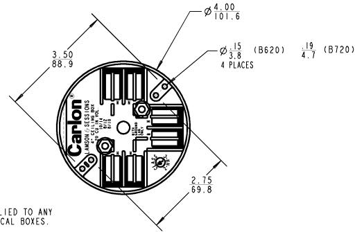
\* SOLVENTS CANNOT BE APPLIED TO ANY POLYCARBONATE ELECTRICAL BOXES.
