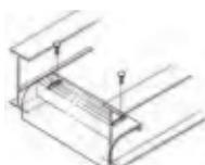
Designed to provide a smooth radius surface at any position on the tray or trough bottom.
