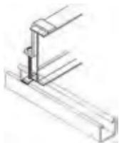
Designed to secure cable tray to support system.
