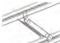
Allows cables to run from one tray level to another.
