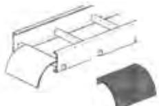
Specially-designed ladder drop-outs provide a rounded surface with adequate radius to protect cable as it exits from the tray, preventing damage to insulation.
