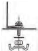
Barrier strip clamps mount barrier strips to ladder rungs and ventilated trough bottoms. Complete mounting hardware supplied.
