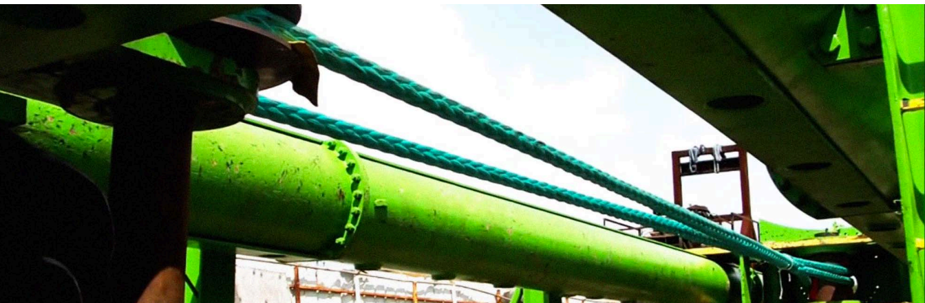
Pictured Below: Break testing of a high-strength 8 braid mooring line.
