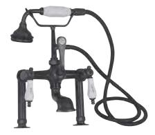
7" centers • Spout length is 5" 1/4 turn ceramic disc cartridges • 59" hose Flow rate 3.7 GPM Flow rate handshower 2.5 GPM
