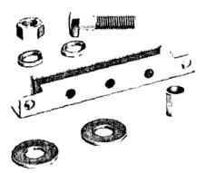
The chain tensioner frame may be mounted on surfaces parallel to or at 90° to the plane of the chain drive. Mounting is accomplished by using two 5/16" dia. bolts, provided by the user. Parallel surface mounting provides a full 4" of adjustment. Installation on a surface 90° to the chain drive, will limit adjustment to  $2\frac{1}{2}$ " or  $1\frac{1}{2}$ ", depending on which intermediate mounting hole is used.
