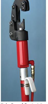
Hydraulic ram fully retracts in the Open position. For efficient cutting, upper and lower jaw edges are sharpened.
