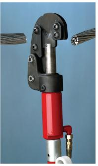
Hook-style jaw hangs on conductor to help position tool. Guillotine-type blades result in smooth, clean cuts.
