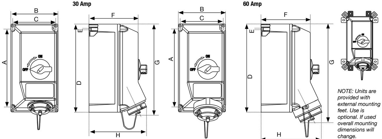
NOTE: Units are provided with external mounting feet. Use is optional. If used overall mounting dimensions will change.
