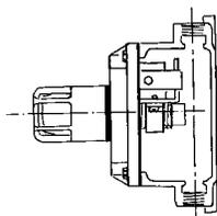
Add Suffix as listed below. Transformer clamps directly to pilot light barrel. **Only one pilot light transformer assembly per one gang body.**
