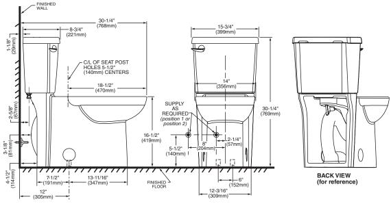
IMPORTANT: Water supply on the wall is required at 2-1/4" or 8" from centerline of the toilet (see rough-in). First suggested position is hidden behind the toilet. The geometry of the toilet gives pace for this installation. The second suggested position is next to the toilet. Between these two positions, the space for the supply between wall and toilet is limited to 4-1/2". In this case, check your supply and hose dimensions.
