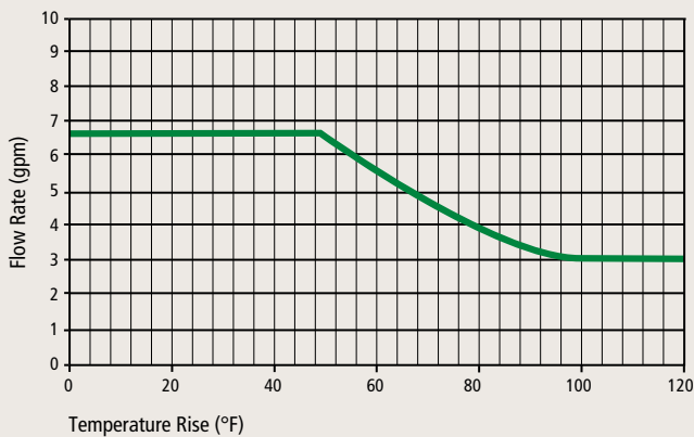
240H: Flow Rate vs. Temperature Rise
