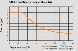
Set Temperature 130°F (55°C) or higher, maximum flow rate is limited to 8.0 gpm.
