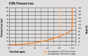
Set Temperature 125°F (52°C) or higher, maximum flow rate is limited to 8.0 gpm.
