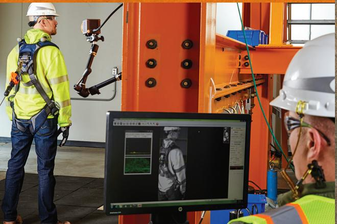
How did we create an SRL that reduces unintentional lockups? Using advanced motion capture technology, 3M studied the way users work, move and interact with SRLs on a typical job site. This data helped us engineer an arrest mechanism designed to better accommodate your natural work motions—resulting in fewer unintentional lockups.\*
