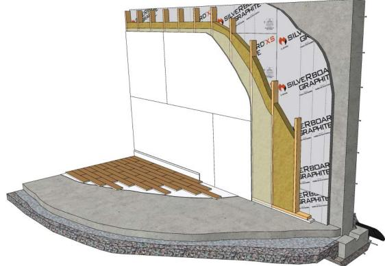
Typical foundation wall assembly with SilveRboard installed on the interior
