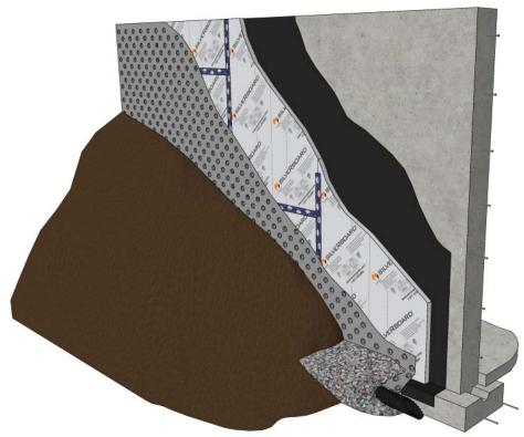
Typical foundation wall assembly with SilveRboard installed on the exterior
