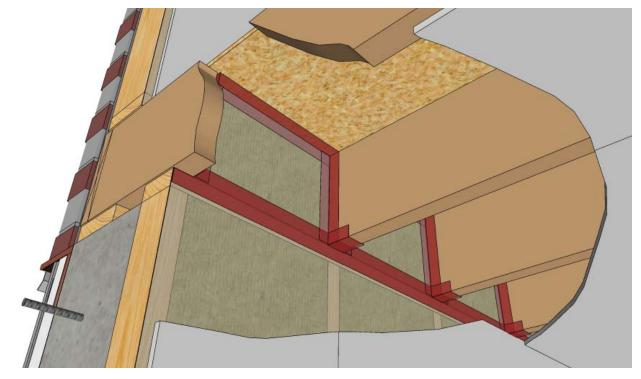
Rim joist at foundation detail
