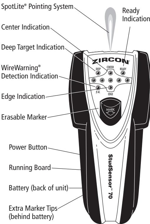
The Zircon StudSensor™ 70 detects both the center and edges of wood and metal studs and joists in walls, floors, and ceilings in one step. It features a durable high-impact case and patented SpotLite® Pointing System.
