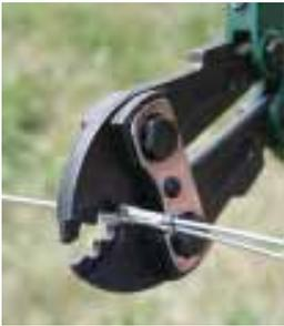
HTGCS1225    | Crimping Sleeve 1-2      | Use to splice 14½ & 15½ gauge wire. Use crimping tool (model 300-320) to crimp and hold lines together, packed in a pegable bag.                                                                                    | 10 bags per carton, 25 per bag             |
