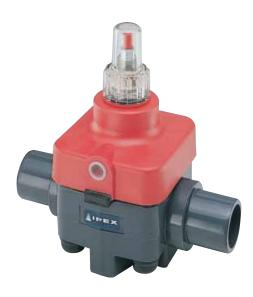
Diaphragm valves are the perfect solution when precise flow throttling is required. The weir style design - no dead space in the valve - is extremely good for abrasive slurries. These valves are widely used in high purity applications because their design prevents friction and subsequent particle creation when cycling. Many body and diaphragm material options are available as well as simple pneumatic actuation.
