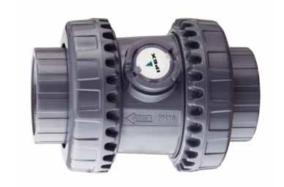
With optimized fluid dynamics design the SXE has an improved Cv value. The seat stop carrier is a threaded design for safe disconnection upstream. The ball is machined smooth for optimal service and prolonged life. The SXE also utilizes the EASYFIT torque wrench to tighten union nuts with defined torque and the EASYFIT LCE labelling system for custom identification.
