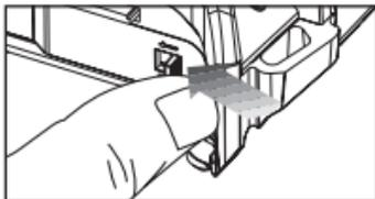
3. With the bottom of the camera towards you, Make sure to insert the batteries into the camera with the positive ends towards you where marked positive and the negative ends towards you where marked negative.
