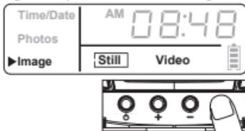
2. Press the + or - navigation button to move to different options. Press the enter navigation button to save the setting.
