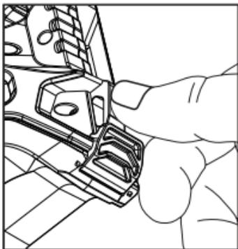
2. With the camera facing open, open the battery compartment cover by sliding the latch to the left.
