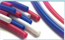
Sea Tech tubing is produced from a high performance, crosslinked Polyethylene material. Sea Tech tubing is formulated and manufactured in 1/2" CTS (5/8" O.D.) size. Sea Tech tubing is NSF listed, FDA recognized and available in multiple colors for ease of water line identification.
