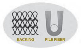
Both the backing and the pile fibers are different in knit and woven fabrics. In simple terms, knitted fabrics have a looped backing, and the pile fibers are secured to the backing with a single pass-through. The resulting fabric is more "open" than a woven, so it can pick up and release more paint for the fastest coverage. Knit rollers are recommended for flat, eggshell, or satin paints and stains.
