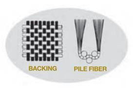
Woven fabrics have a backing with a tighter cross section. The pile yarns are made with a twist that helps lock the fibers into the backing, and they are secured using two pass-throughs. This "double lock" process results in a shed-resistant fabric that provides the smoothest, virtually lint-free finish. Woven rollers can be used with confidence in enamels, primers, and all paints: flat, eggshell, satin, semigloss, and gloss.
