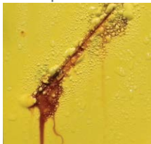
Metal panels after 240 hours of salt-fog exposure.
