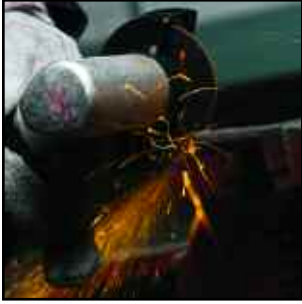
Cutting a piece of steel tubing to length.
