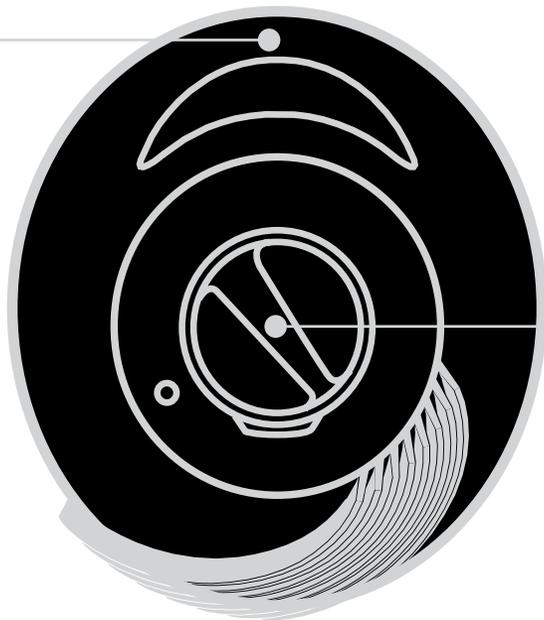
4. Select Mode by turning control dial. In Fan Only
