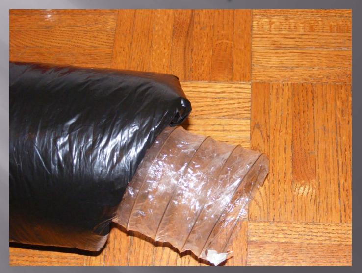
Secure the duct onto the exhaust pipe with a good quality duct tape and clamp, making sure it is completely air tight.
