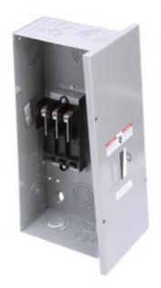
Siemens Energy Management Residential Specialty Load Centers: Small Circuit (2-10). Sub Brand: Load Centers Type: 1: Application: Residential: Voltage Rating: 120/240V Amperage Rating: 60A Phase: 1PH Load Regulation: 60A Wiring Configuration: 3w Bus Rating: 60A Interrupt Rating: 100000AIC. EQ LC 2S 4C ML 60A N1-S DIY
