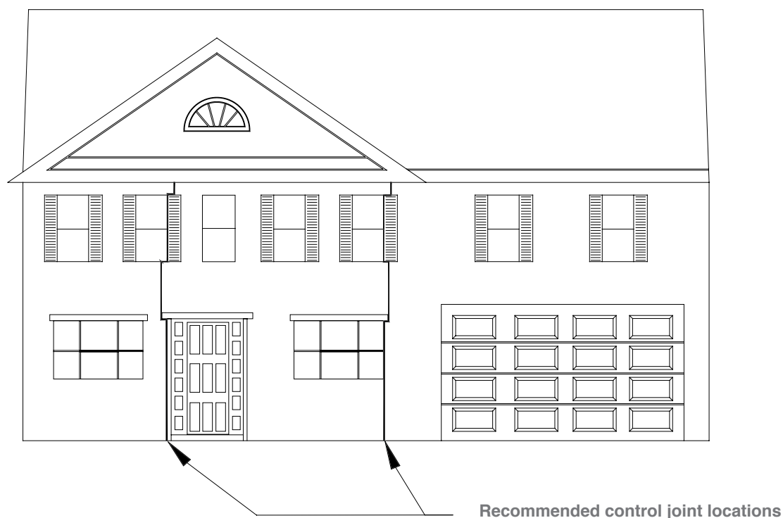
Figure 2 - Example of Residential Control Joint Placement
