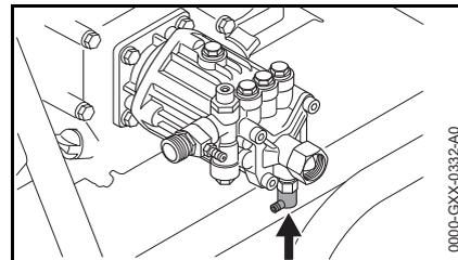
If the engine is running in standby mode without active spraying, the water in the high-pressure pump heats up to 60 °C (140 °F). The thermal pressure relief valve automatically lets the hot water escape from the high-pressure pump so that fresh and cool water can flow into the system.
