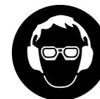
To reduce the risk of eye injury, always wear goggles that are impact-rated and marked as complying with ANSI Z87 "+". Wearers of prescription (Rx) eyewear should wear goggles that can be worn over prescription lenses without disrupting either the prescription eyewear or the proper fit of the goggles.
