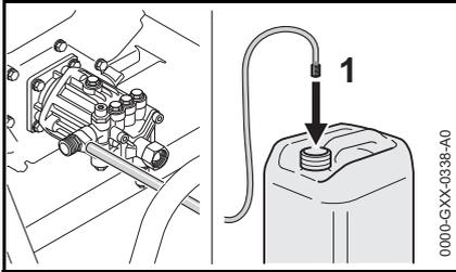
Use the detergent suction hose to draw detergent from a separate container. The detergent is added to the water in the high-pressure pump:
