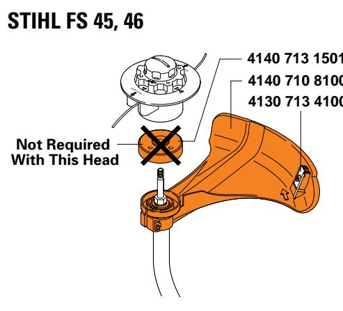
**Semi-automatic, dual line cutting head for trimmers**
