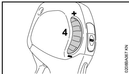
The thumb wheel (4) is used to set the throttle path infinitely between idling and full throttle and therefore also the engine speed range:
