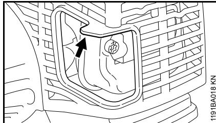
The spacer (arrow) is integrally molded to the shroud.
