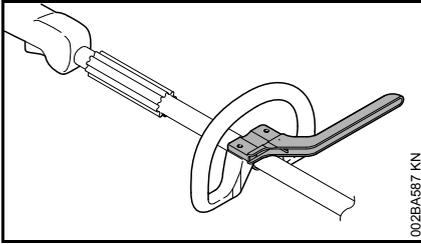
The barrier bar comes standard with the machine and must be mounted to the loop handle.
