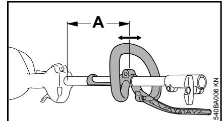
The loop handle can be adjusted to suit the height and reach of the operator and the application by changing distance (A).
