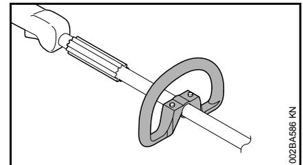
A factory-new machine comes with the loop handle already mounted.
