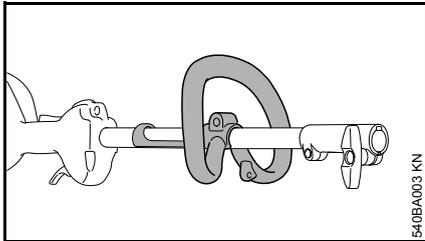
A factory-new machine comes with the loop handle already mounted.
