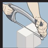
**TIP 9** With all types of cut support the waste material as you near the completion of the cut.
