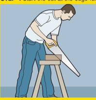
the saw cutting edge angled at approximately 30° to the work surface. Use the thumbnail of the hand not holding the saw, or a scrap piece of wood, position the cutting edge to the waste side of the line. The first stroke should be a light pull to establish the cutting line (kerf).
