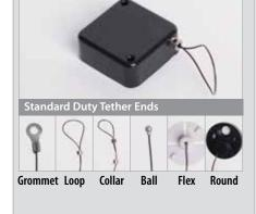
Box dimensions: 1.875"W x 1.875"L x .625"H Cable dimensions: 36" long x .032" dia. nylon coated aircraft cable
