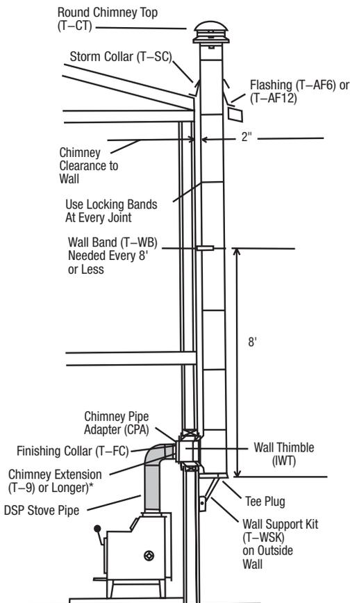
\*The end of the chimney section must extend into the room a minimum of 4-1/2" beyond the face of the wall.
