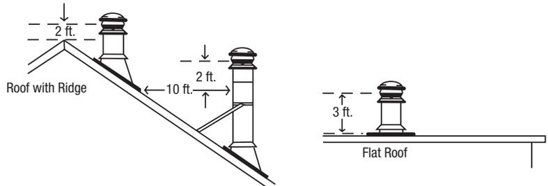
The chimney must extend at least three feet above the highest point where it passes through the roof surface and at least two feet higher than any part of the building within a horizontal distance of ten feet.
