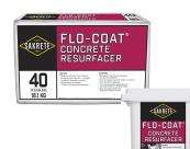
Sakrete<sup>®</sup> Flo-Coat<sup>®</sup> Concrete Resurfacer is a polymer modified concrete resurfacing material requiring only the addition of clean potable water. For resurfacing concrete substrates. Can be applied in a flowable consistency using a squeegee, in a stiffer consistency using a trowel or can be sprayed through a hopper gun
