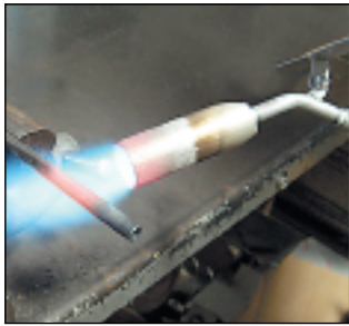
The HT torch is great for heating flat iron or metal tubing.
