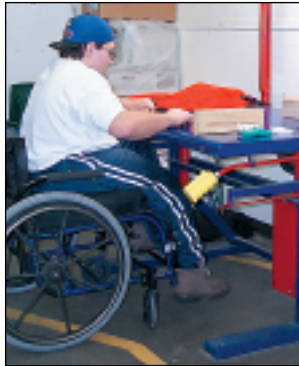
The SP-34 Bench provides plenty of leg room and height adjustment at the push of a button.
