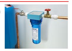
Featuring full ¾" threaded ports, the FC100 system can be installed on ¾" or ½" copper or PEX pipe, after the water meter or pressure tank, depending on the water supply.
