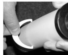
If gauge does not pass over the cartridge
