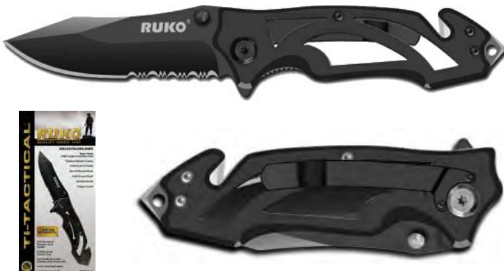
RUK0165: locking liner rescue folding knife, black titanium nitride coated 50/50 serrated drop point blade and vented handle; ambidextrous thumb studs; window punch and seat belt cutting blade; reversible low rise pocket clip, blade: 3-3/8" closed: 4-3/4" boxed RUK0165-CS: as above clamshell packaging
