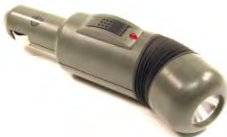
JL-04: rechargeable auto light, charges through 12V accessory socket, flexible head, ABS housing, Krypton Bulb
