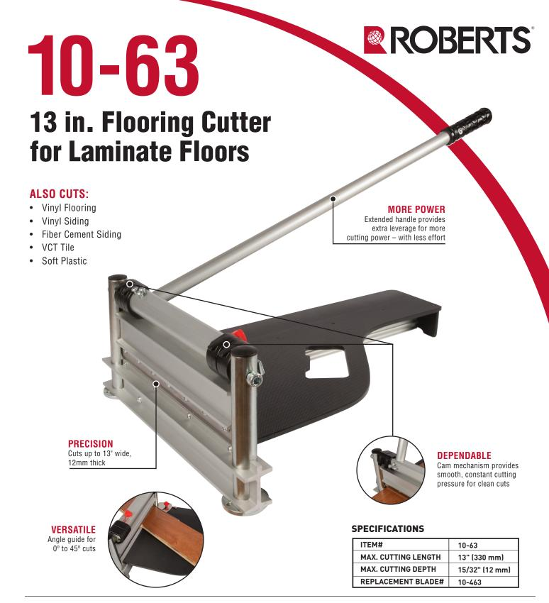
The 10-63 13 in. Flooring Cutter will easily cut laminate planks up to 12mm thick. The cam mechanism provides smooth, constant cutting pressure for clean cuts while the extended handle gives extra leverage for more cutting power. It's quiet, dust free and electricity free operation means that flooring can be cut on the site of the installation and job cleanups are easier. The 10-63 is perfect for cutting end pieces to be covered with base moldings.
