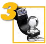
Using a Reese Towpower Hitch Ball Wrench, tighten the InterLock Hitch Ball nut to specifications (See Hitch Ball Package)
