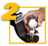
Place the Hitch Ball shank through the hole of the Ball Mount. Align the hex shape of the Hitch Ball platform so that it fits into the hex recess of the Ball Mount
