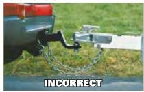
Sometimes a trailer's tongue is higher or lower than the ball mount on the vehicle, and a ball mount with a "rise" or a "drop" is required to level the trailer.
