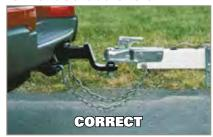
For safe, comfortable towing, the trailer should always be set up to tow on a level plane.
